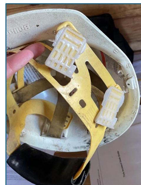
Top – FAL1's helmet showing external damage to its shell. Bottom – FAL1's helmet showing its internal damage.
